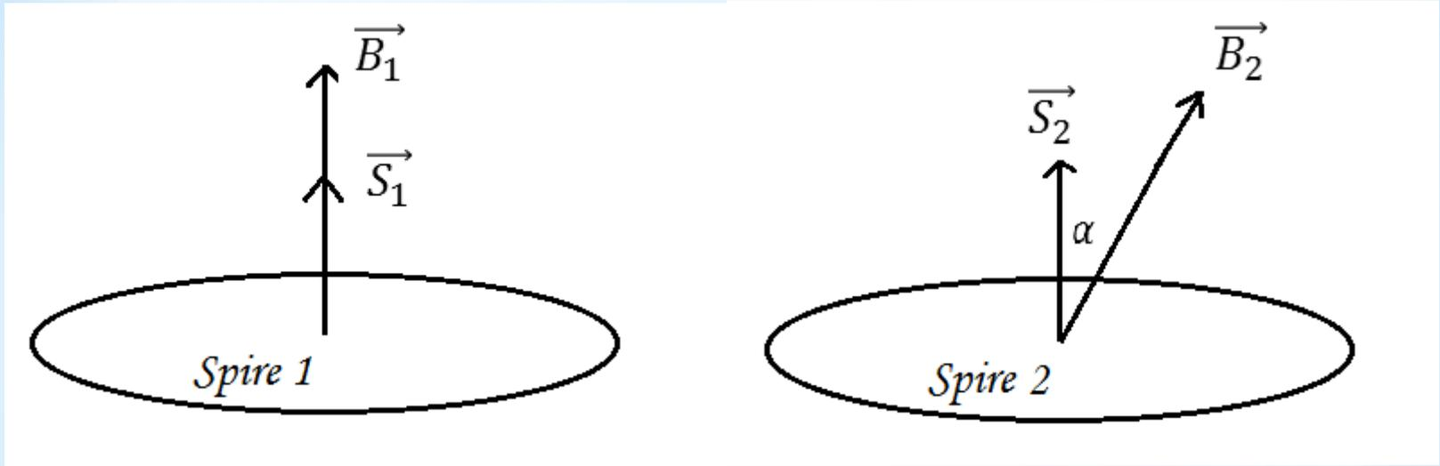
$$\varphi_1 = N \times B_1 \times S_1 \times \cos 0 = 1 \times 0.08 \times 10 \times 10^{-4} \times 1 = 8 \times 10^{-5} \text{ (Wb)}$$
